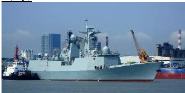
The Type 054A/P Pakistan-specific variant equipped with the SR2410C long-range and Type 517/SUR17B air-surveillance radars. Photo: Pakistani Government
